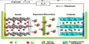
Figure 3.Charging working principles of Lithiumion battery
