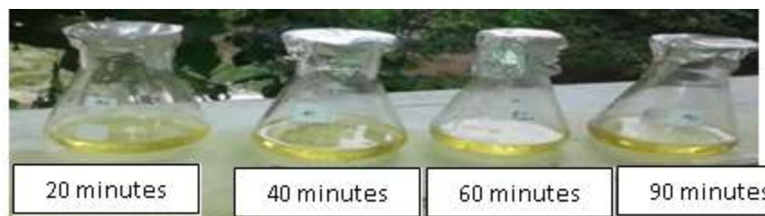
Figure 5. Effect of contact time on the purity of WCO
