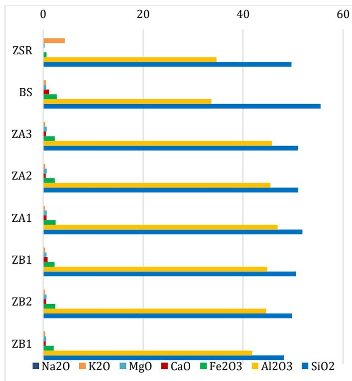
Figure 3. XRF characteristics of zeolite products (x axis = %) using NaOH (ZA) and  $Mg(OH)_2$  (ZB) as reactants in various concentration (1, 2, 3 = Molar) in comparison to brick sample (BS) and synthesized zeolite from reference (SZR).
