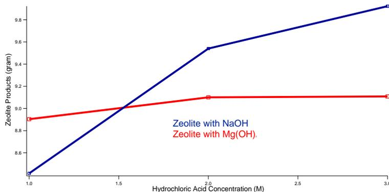
Figure 2. The effect of HCl concentration on yielded zeolite using NaOH and  $Mg(OH)_2$  as the reactants
