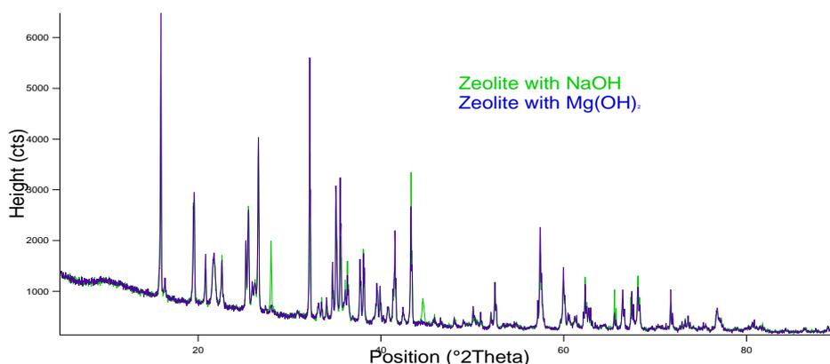
Figure 4. Overlaid XRD diffractogram of zeolite products using two different reactants.
