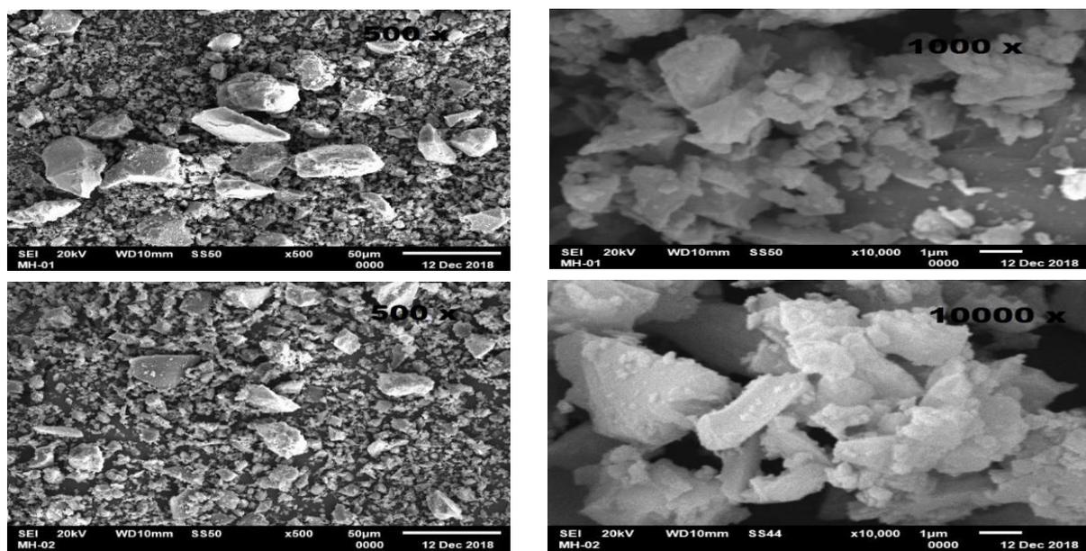
Figure 5. SEM images of zeolite products with different reactants, NaOH (left) and Mg(OH)<sub>2</sub> (right)
