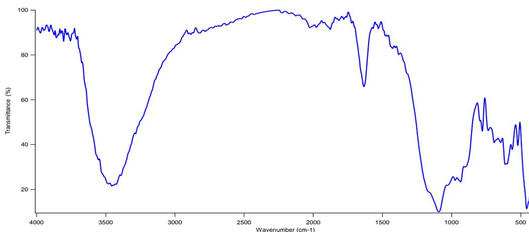
Figure 1. Infra-Red spectra of synthesized zeolite
