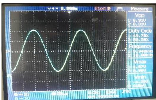
(b)  $F = 10 \text{ kHz}$  dan  $V_{pp} = 8.31 \text{ V}$
