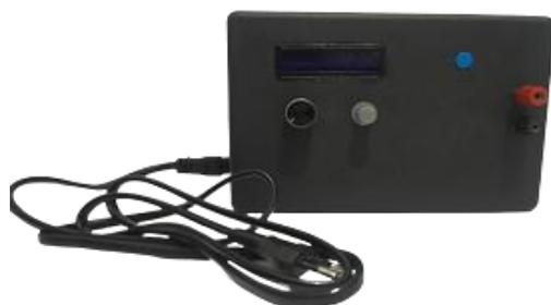
Gambar 5. Realisasi Rancang Bangun *Voltage-Controlled Oscillator* (VCO) Multifrekuensi (10kHz – 1MHz)
