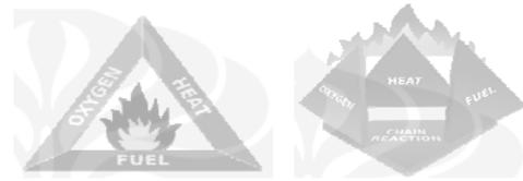
Gambar 1 (a) *Fire Triangle* (b) *Tetrahedron of Fire*
