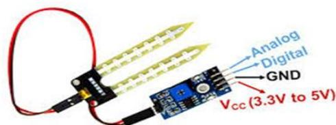
Gambar 2. Sensor Kelembaban Tanah
