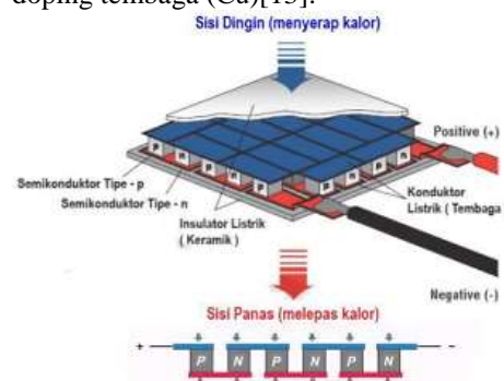
Gambar 1. Elemen Peltier ( Thermo – Electric Cooler ) dan Cara kerja peltier [13].
