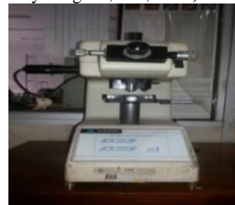
Gambar 3. Alat uji kekerasan merk Buchler Micromet 2100 Series
