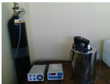
Gambar 3 Kalorimeter *bomb* Toshiwal Ltd.
