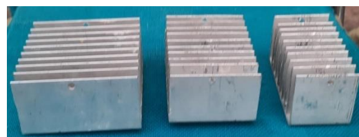
Gambar 2. Heatsink bersirip 4 cm, 6 cm, dan 8 cm.
