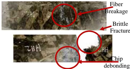
Fig. 4 Damage of DCFC (Feraboli et.al, 2009)
