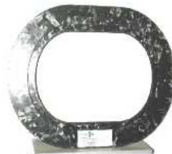
Fig. 1 Window frame of Boeing 787 Dreamliner (Turtle et.al, 2010)
