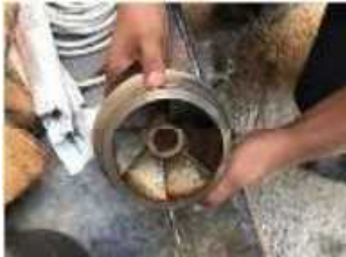
Gambar 4. Impeler Pompa Air Boiler
