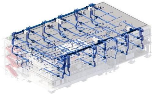
**Gambar 9.** Isometri Sistem Penghawaan
