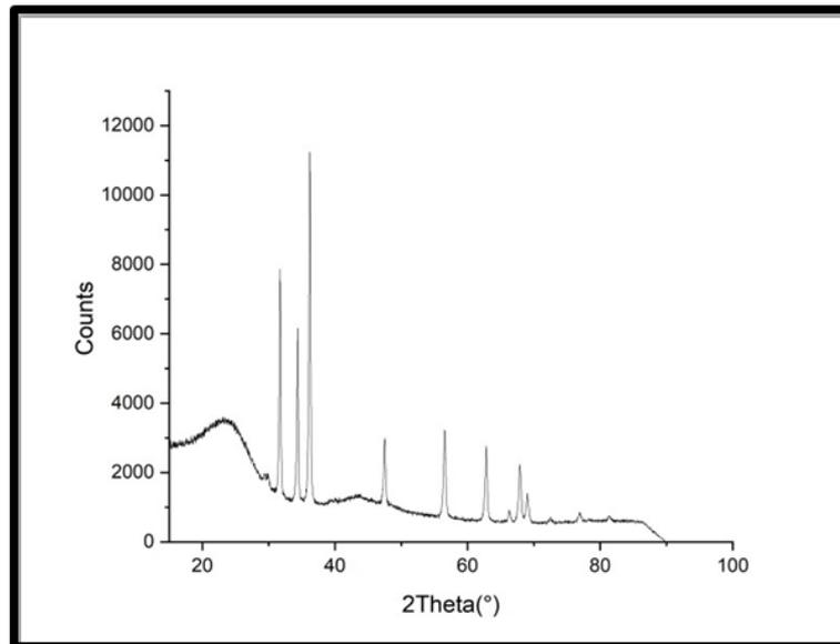
Figure 1. X-ray diffraction pattern of the AC/Zn
