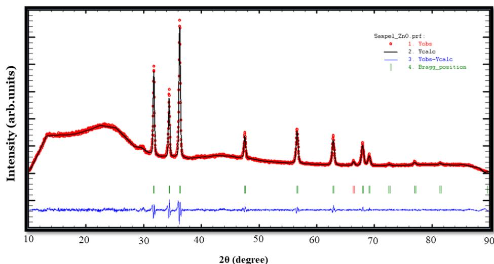
Figure 2. Rietveld refinement pattern of the AC/ZnO composite
