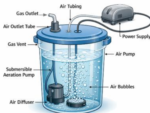
Figure 1. Schematic diagram of the aerobic reactor system
