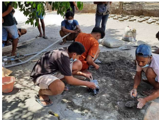
Gambar 2. Proses mencetak paving block
