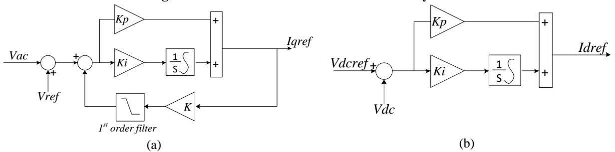
Figure 3. PI Controller of STATCOM system, (a)  $I_{qref}$  loop, (b)  $I_{dref}$  loop
