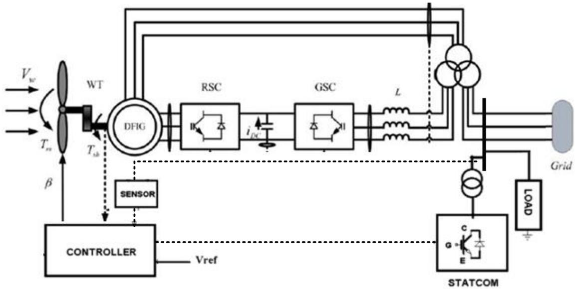
Figure 1. Schematic diagram of the wind generation system
