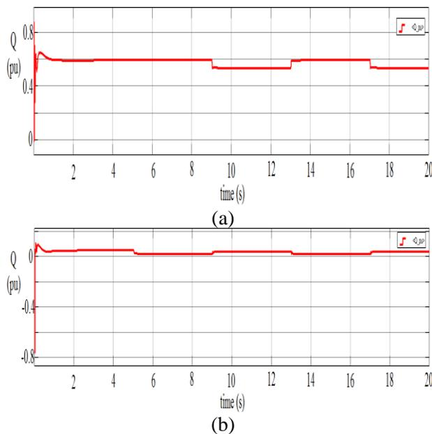
**Figure 4. Reactive power flow with resistive load (a) without STATCOM and, (b) using STATCOM**
