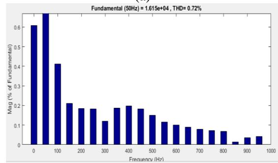
**Figure 7. THD of resistive load (a) without STATCOM and (b) using STATCOM**
