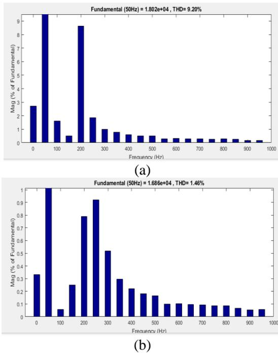
**Figure 9. THD of capacitive load (a) without STATCOM and (b) using STATCOM**
