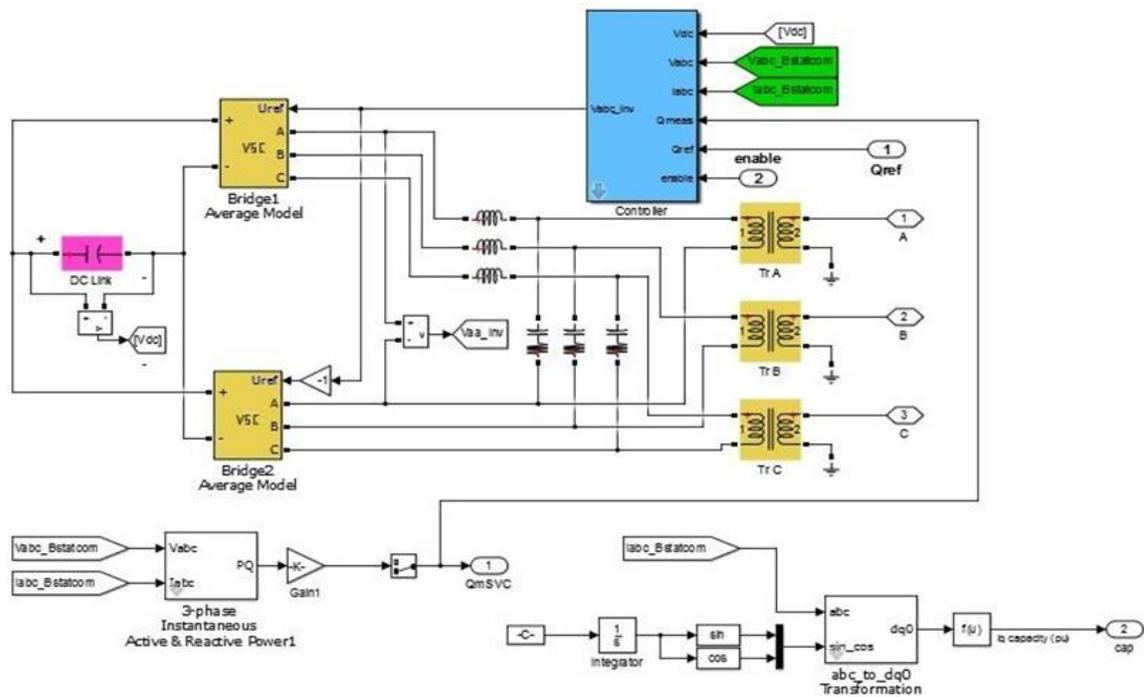
Figure 2. Schematic control of the STATCOM system
