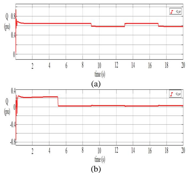
**Figure 5. Reactive power flow with inductive load (a) without STATCOM and (b) using STATCOM**
