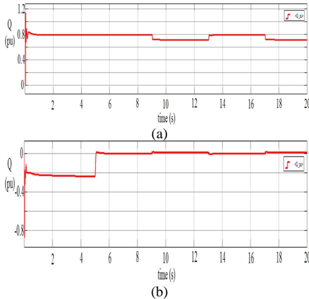
**Figure 6. Reactive power flow with capacitive load (a) without STATCOM and (b) using STATCOM**
