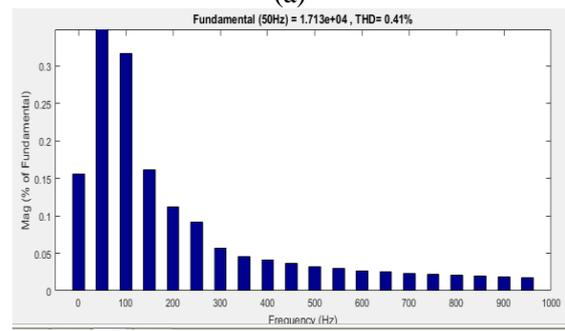
**Figure 8. THD of inductive load (a) without STATCOM and (b) using STATCOM**
