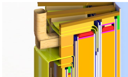
Figure 1 Typical Insulation Arrangement in Power Transformer
