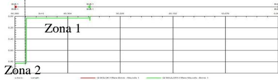
Gambar 3.2.b Kurva Time Distance Rele Impedansi Maulafa – Bolok (Baru)
