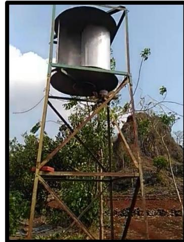
Gambar 3. Turbin Savonius
