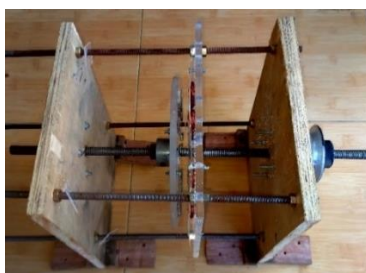
Gambar 4. Generator Aksial Magnet Permanen
