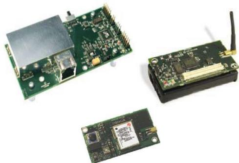
Gambar 3. Gateway (MIB 600), Micaz Mote (MPR 2400) dan Sensorboard (MTS420) [5]
