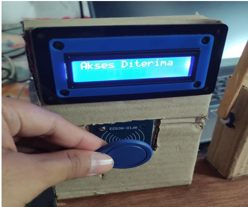
Figure.14 Scanning RFID tags on RFID reader
