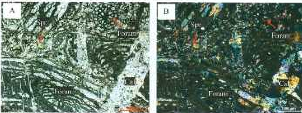
Foto 5. Fotomikrograf sayatan tipis no. lab. 2199/21, kode: 05/OT/PF/2022; [A] nikel sejajar, [B] nikel bersilang. Ket.: Cal= Kalsit, Foram= fragmen foraminifera besar, Spr= sparit.
