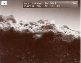
Fig. 6. SEM micrograph of the (a) Support, (b) Membrane (surface) and (c) Membrane (cross section)
