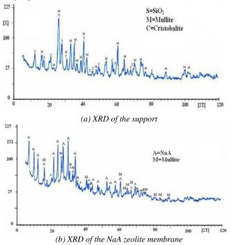
Fig. 5. XRD of the (a) Support and (b) NaA zeolite membrane
