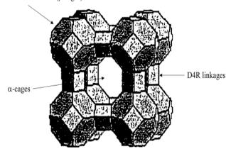
Fig. 1. Repeating unit of the zeolite NaA
